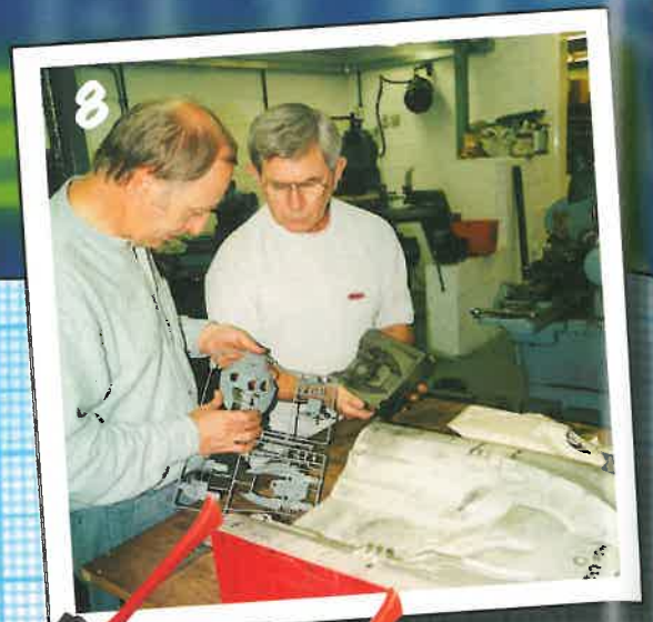
Stage 8: Tool makers Terry and Bob check the first test sprues against the resin for accuracy and to make sure the detail shows correctly
