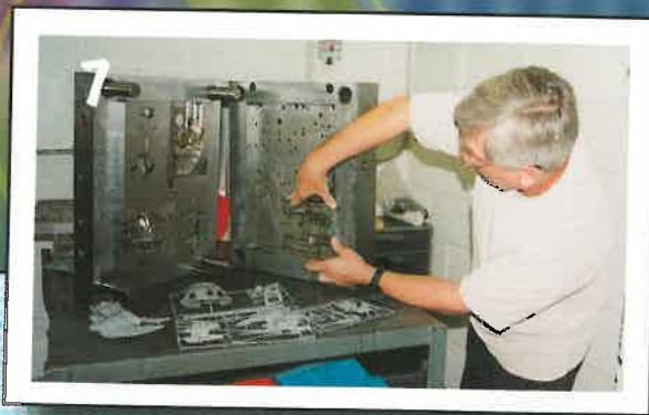
Stage 7: The finished steel moulds for each component are then mounted into a die so the first test sprues can be produced.
