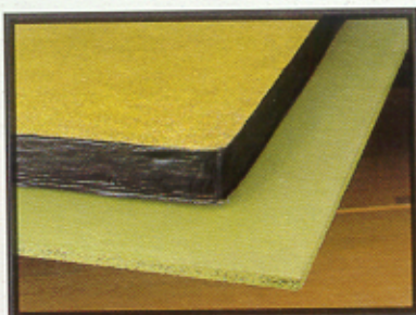
▲ Two gaming boards made from a thick sheet of polystyrene (top) and chipboard (bottom).
