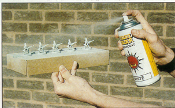
▲ Spray your models in a well ventilated area, preferably outdoors. If you place your models on an upturned box you can rotate them and spray the other side without having to touch them.
